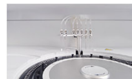
Washing Probe Independent 7-step washing system.
