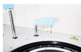
Mixer Probe Teflon coating to avoid cross contamination.
