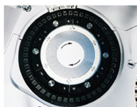
Reaction Tray 37±0.2°C, real-time monitor.
