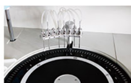
Washing Probe Independent 7-step washing system.
