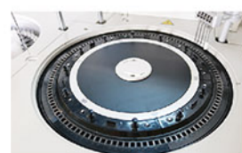
Reaction Tray 37±0.1°C, real-time monitor.
