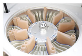
Reagent Tray 2~8°C cooling for 24 hours.
