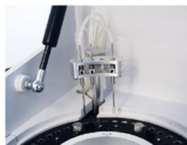
Washing Probe Independent 3-step washing system.
