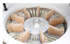
Reagent Tray 2~8°C cooling for 24 hours
