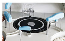
Reaction Tray 37±0.1°C, real-time monitor.
