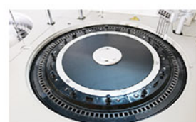
Reaction Tray 37±0.2°C, real-time monitor.
